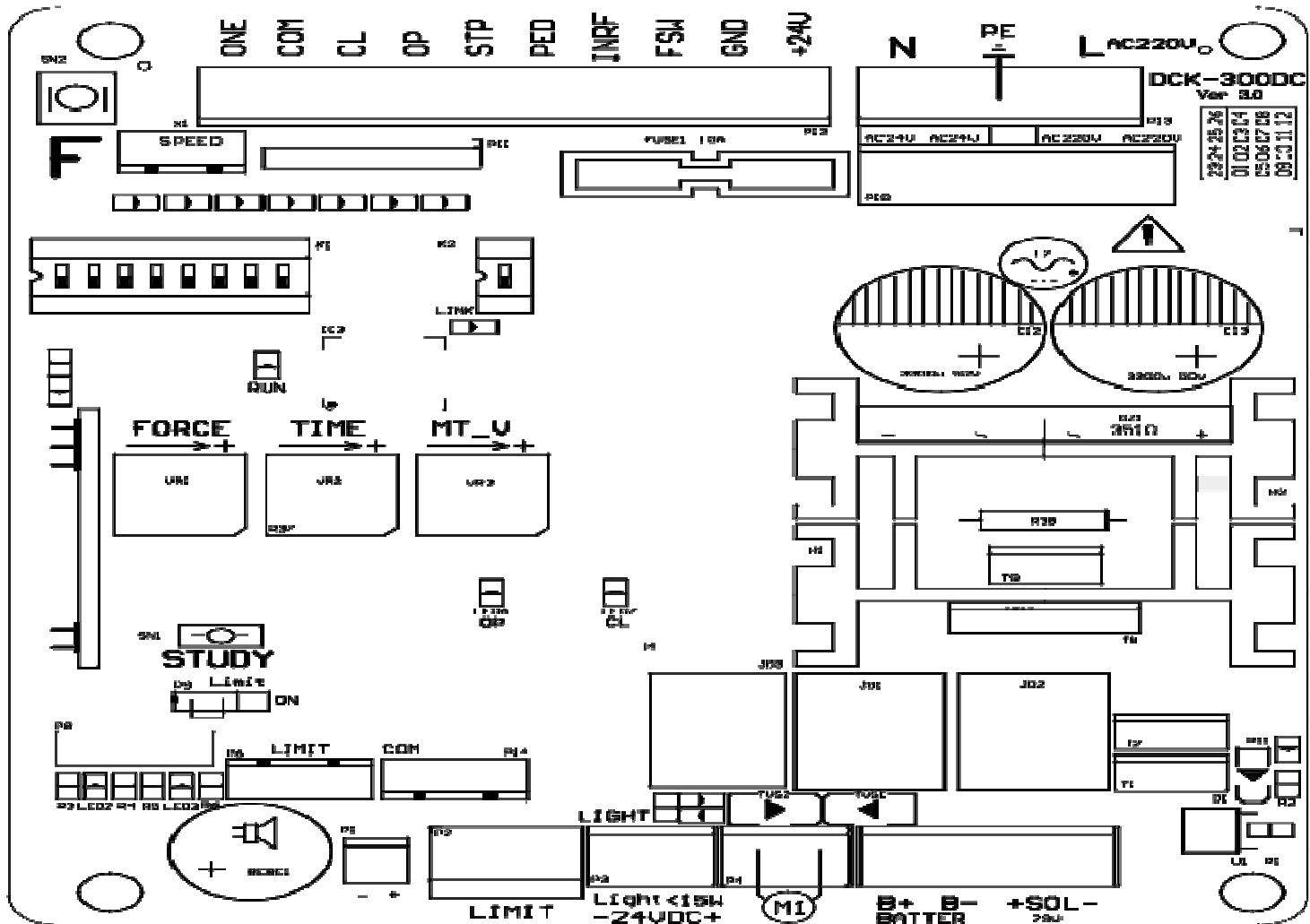
When the door is in the closing motion, the infrared sensor FSW detects an input. The door stops and immediately rebounds to the open position to prevent any obstructions.
